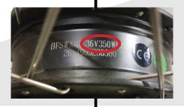
If the motor hub has "24V" or "36V" etched on it, then it is compatible with the URB. You will need the Universal Replacement Battery, 36V URB Charger, and 36V URB cable set.
