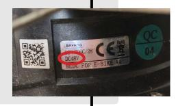
If the motor hub has a "48V" sticker on it, then it is not compatible with the URB. However, we do have a Summit Replacement Battery that will work as a drop in replacement for the motor.
