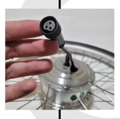
If the connection point looks exactly like this and has 3 holes, then check the voltage and wattage rating etched on the motor hub.
