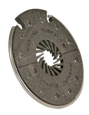
You don't need to remove the crank arm to instal the Magnet Wheel. Removing the metal ring around the magnet wheel allows you to split it into 2 halves for easy installation. When installing the P.A.S. It is important to note that the working surface (labeled on the magnet wheel) of the Magnet wheel is facing the sensor, and the magnets line up with the target logo on the sensor.
