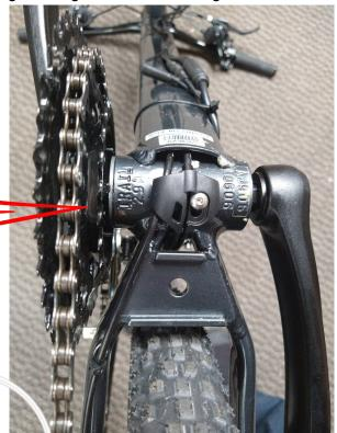
Additionally, the Magnet wheel opening has an inner diameter of **2 cm and can stretch to about 2.5 cm** to fit on the drive side of the spindle shaft, behind the innermost sprocket. The teeth on the opening can fit most spindles, **even square or odd shaped spindles**.
