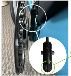
The Pedal Assist System (P.A.S.) is included with some of our kits, like the Horizon and Summit kits. The P.A.S.is designed as another way to give you a boost, along with the regular throttle. It engages when it recognizes that you are pedaling while still under the maximum speed limit. The P.A.S. is optional, and the **kits will still work without it**.
